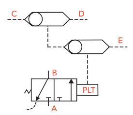
Impulse at C, D or E produces signal from A to B
